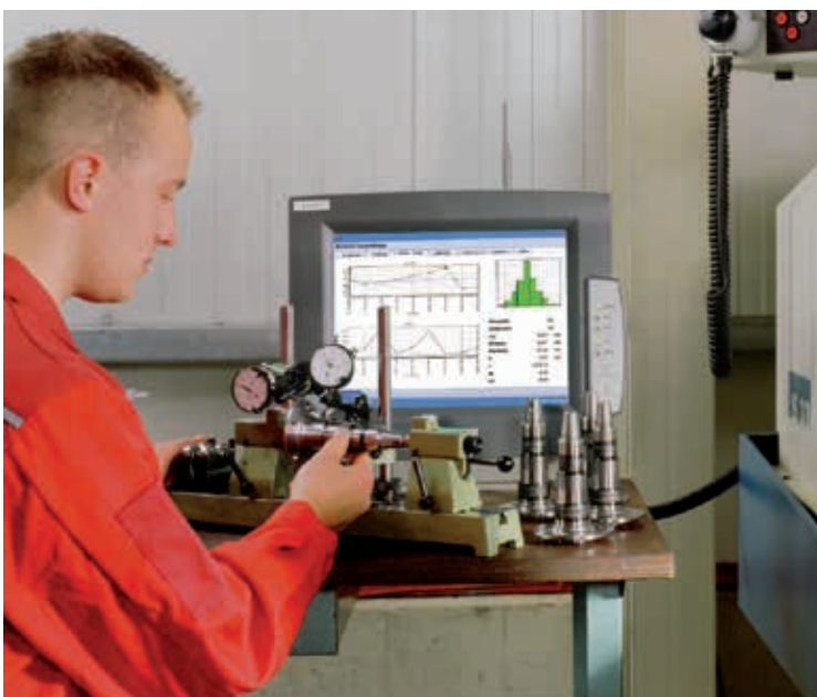
Shop floor data collection and quality management in one system – operator in-production inspection directly at the machine with HYDRA
